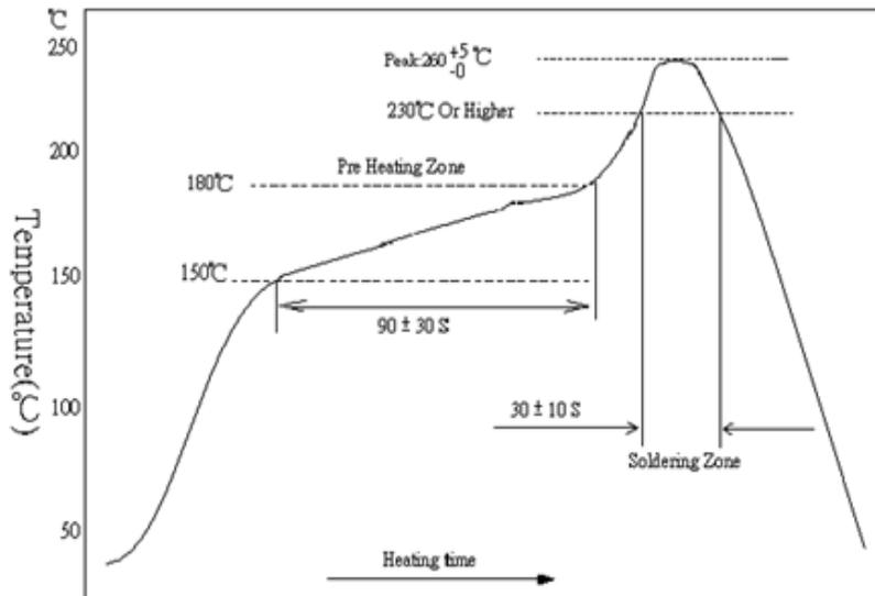
Remark: The peak temperature of soldering heat is  $260 \pm 5/-0$  °C for 10 seconds.
